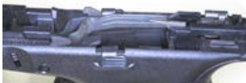
With slide removed the trigger bar can be seen going around the right of the magazine well back to the striker release position.
